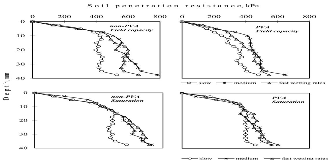
Figure 1. The Effect of Wetting Rate on the Penetration Resistance at 100 kPa Suction of Shepparton Soil
