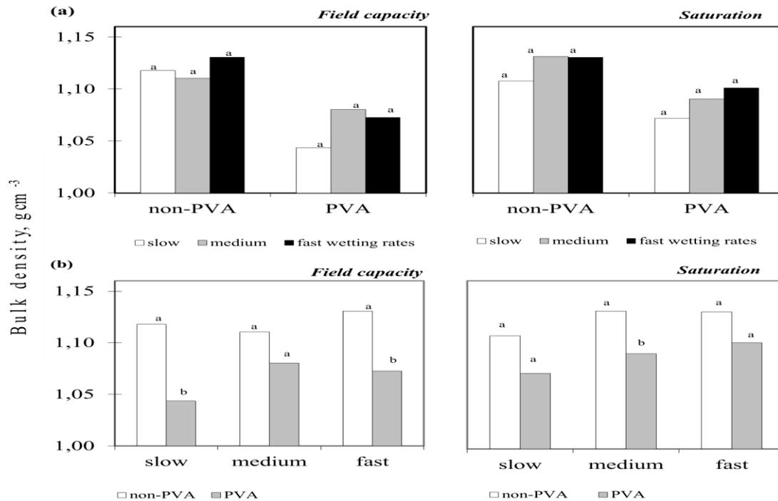
Figure 3. The Effect of (a) Wetting Rate and (b) PVA on Bulk Density at 100 kPa Suction of Shepparton Soil
