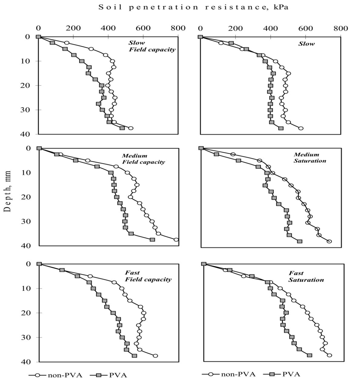
Figure 2. The Effect of PVA on the Penetration Resistance at 100 kPa Suction of Shepparton Soil
