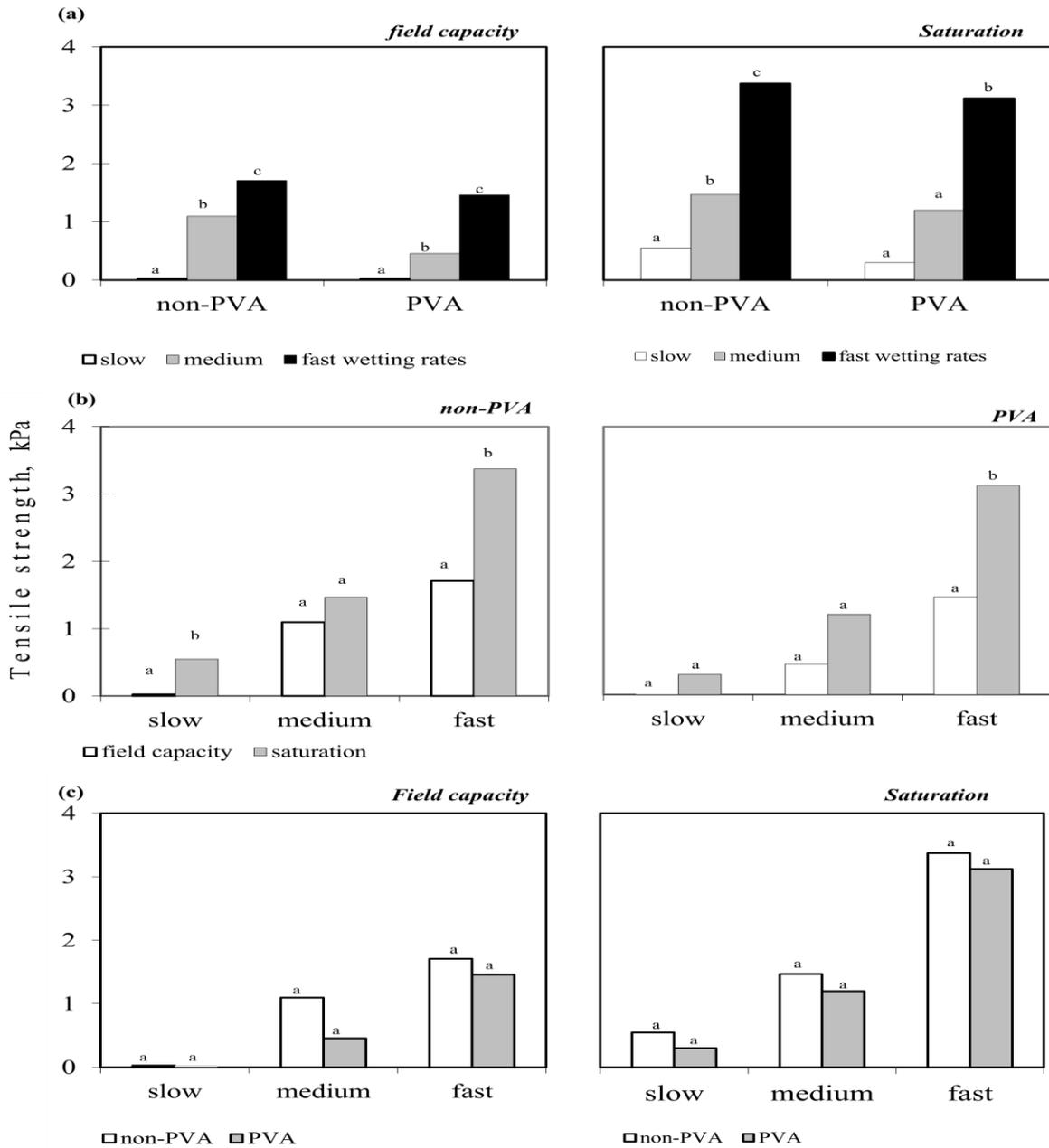
Figure 4. The Effect of (a) Wetting Rate, (b) Wetting Extent and (c) PVA on Tensile Strength of The Air-Dried Shepparton Soil
