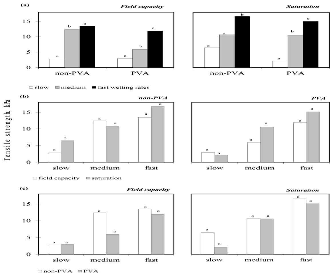
Figure 7. The Effect of (a) Wetting Rate , (b) Wetting Extent and (c) PVA on Tensile Strength of Air- Dried Cornella Soil
