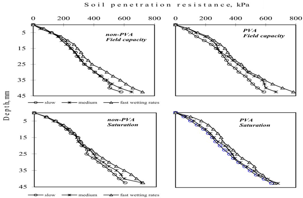
Figure 5. The Effect Of Wetting Rate On Penetration Resistance at 100 kPa Suction of Cornella Soil
