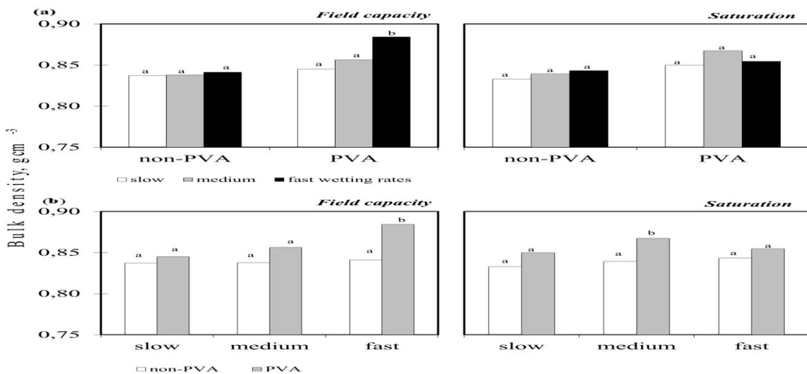
Figure 6. The Effect of (a) Wetting Rate and (b) PVA on Bulk Density at 100 kPa Suction of Cornella Soil
